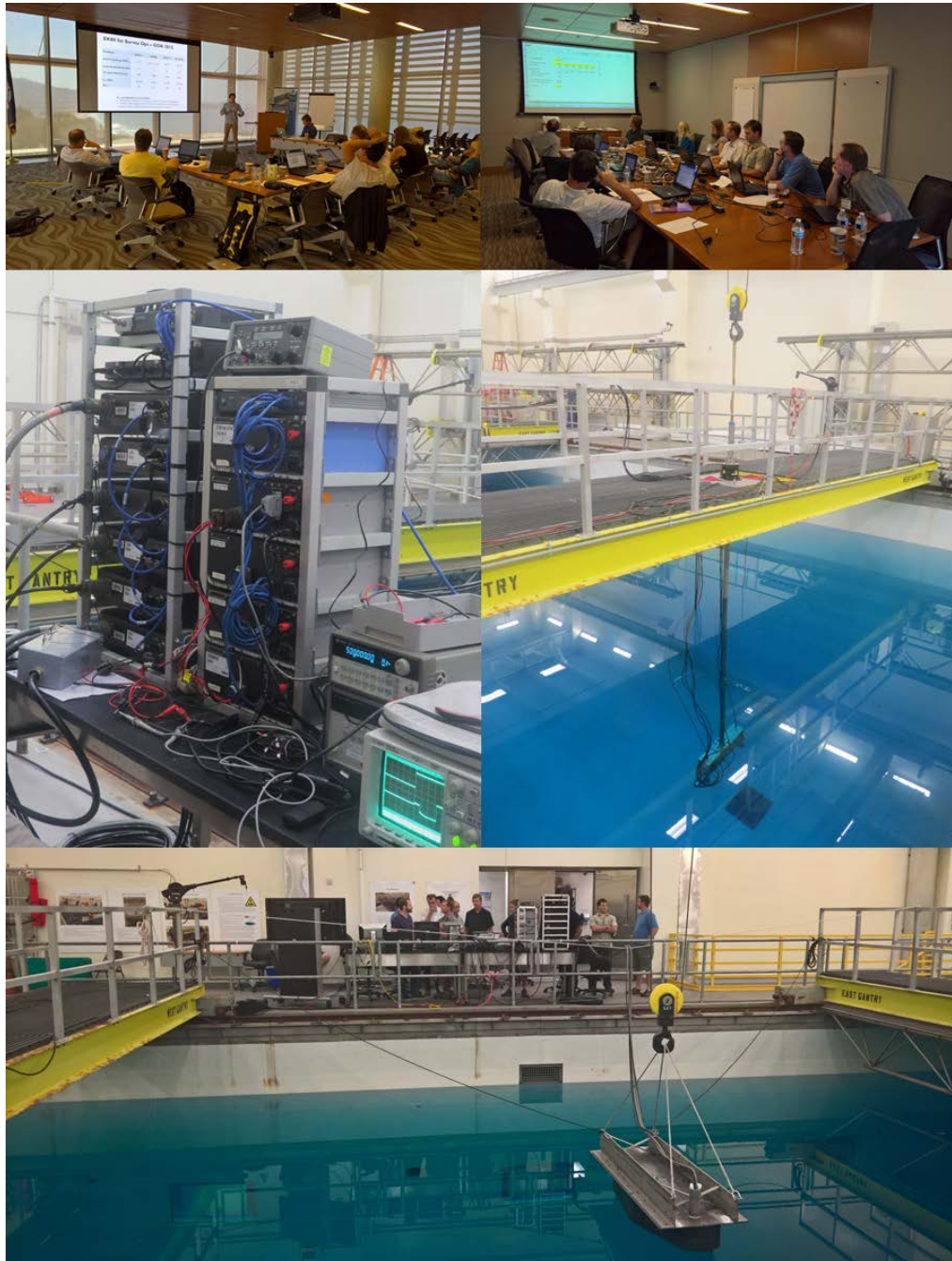
Figure 1. Experimental design, and data collection and analysis activities in Southwest Fisheries Science Center conference rooms (top row) and the Ocean Technology Development Tank during the USA–Norway EK80 Workshop, September 2016. Performances of EK60 and EK80 (middle left) were evaluated and compared systematically using horizontally (middle right) and vertically (bottom) projecting transducer arrays.
