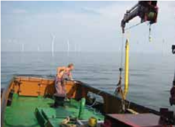
FIGURE 6.5 Deployment of acoustic datalogger (T-POD) outside the Horns Rev Wind Farm.
