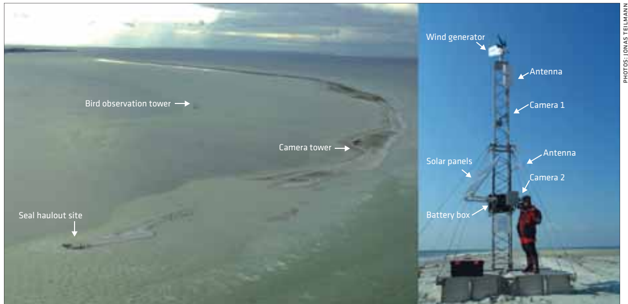
The Rødsand seal sanctuary with the seal haulout site, bird tower and camera tower indicated. To the right a close up of the camera tower.
