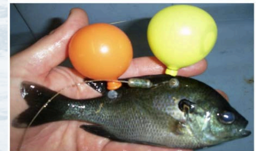
Figure 3-1. Bluegill with HI-Z Turb N' Tags (HI-Z tags) and radio tag attached before (top photo) and after passage (bottom photo) through the HGE hydrokinetic turbine at the Mississippi Lock and Dam No. 2 Hydroelectric Project.
