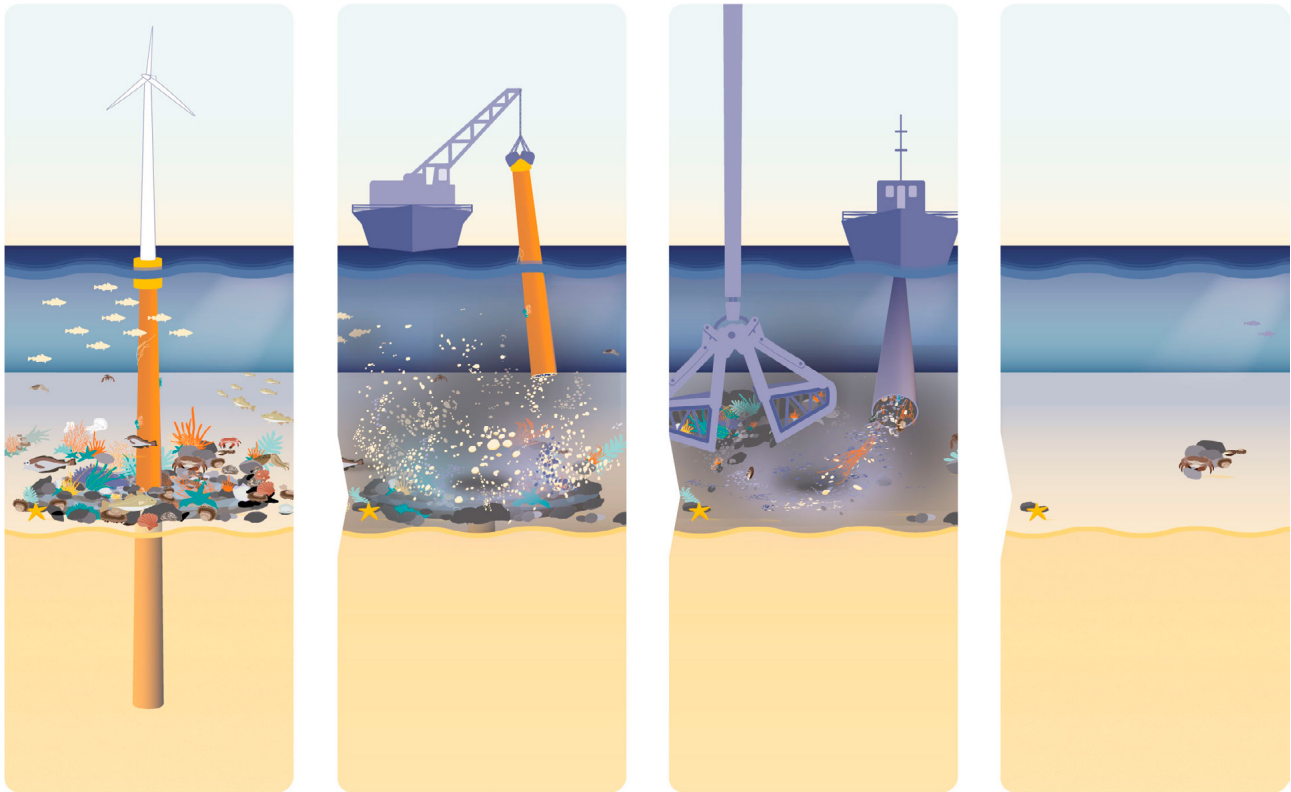
Figure 1: The environmental impact of full decommissioning of an offshore wind turbine
