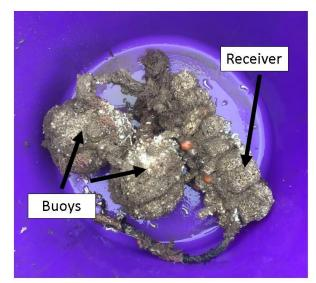
Figure 10. Acoustic tracking receiver and mooring equipment (left); subsurface buoys and receiver after 4 months deployment in the Bristol Channel (right).
