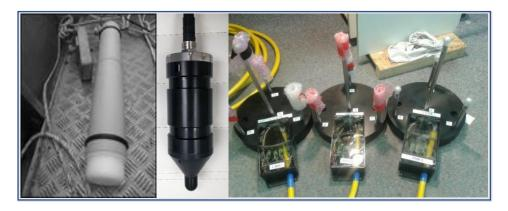
Figure 5. Examples of hydrophone equipment, C-POD (left), SoundTrap (middle, from Copping et al., 2020) and custom-built hydrophone cluster (right, photo taken from Hastie et al., 2018).
