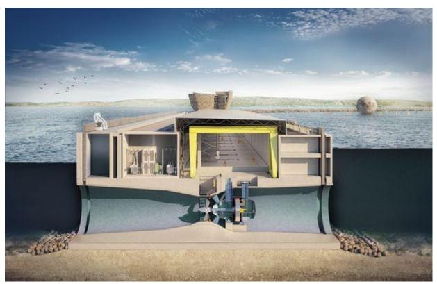
Figure 3. A cross section of the Swansea Bay Tidal Lagoon. Image from Tidal Lagoon Power.
