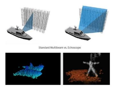
Figure 6. Comparison of standard multibeam coverage versus the Coda Octopus Echoscope coverage (top image), examples of Echoscope imagery (bottom images), taken from Coda Octopus.
