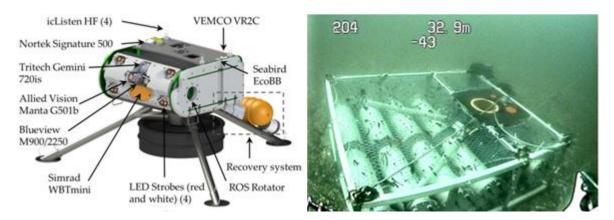
Figure 9. An example of an integrated monitoring system as described in Polagye (2020) on left, and image of the FLOWBEC subsea frame deployed at EMEC tidal energy site from Williamson et al. (2016).
