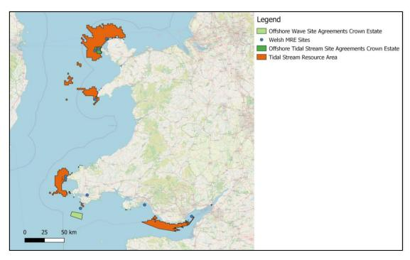
Figure 1. Map of tidal stream energy resource (from LLE portal) with existing and proposed tidal and wave MRE (Marine Renewable Energy) sites and licensed test areas around Wales (data from UK marine energy database and Crown Estate).
