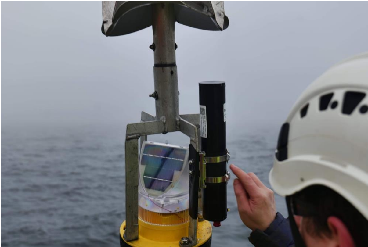
Figure 9 - Automatic bat detector mounted on a buoy used for the marine mammal survey.
