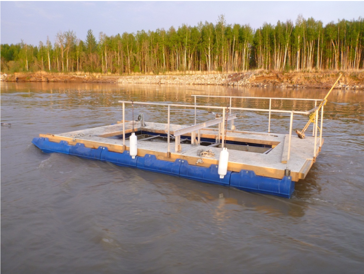
Figure 40. Inclined-plane trap used for sampling the top 1.1 m of the mid-channel of the Tanana River at Nenana, Alaska.
