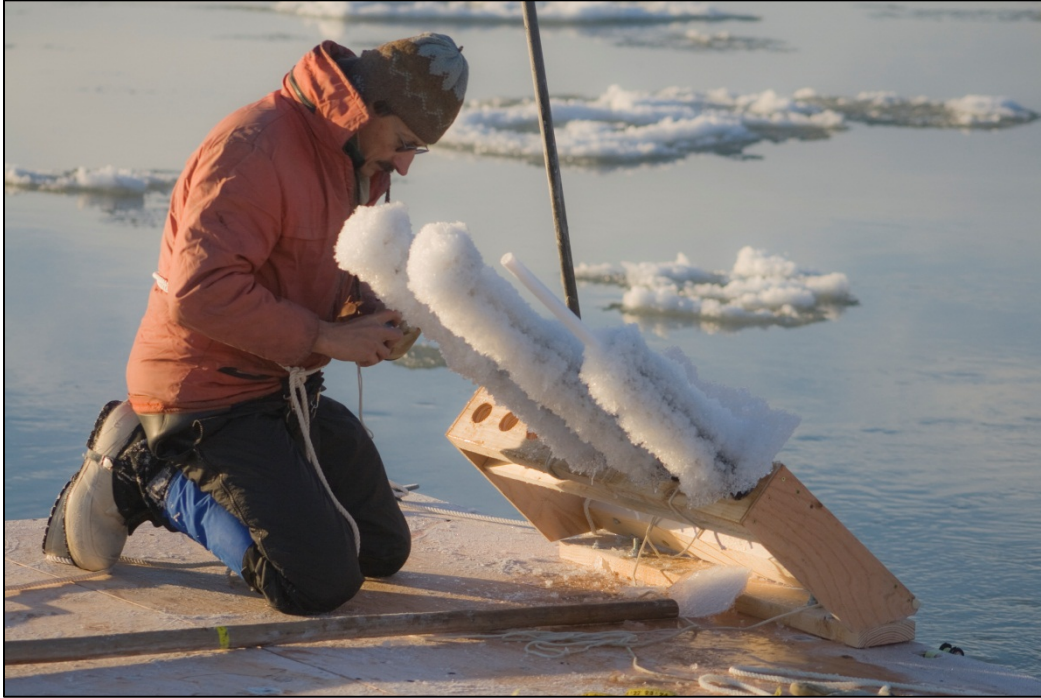
Figure 15. Frazil ice growth on three different materials. From right to left: Teflon ® , 316 SS, and mild steel (Oct. 22, 2010, air temperature = -11°C; 12 hr 40 min of submersion). Frazil growth perpendicular to the current was limited by river shear that eroded the frazil causing the growth to proceed upstream and downstream.
