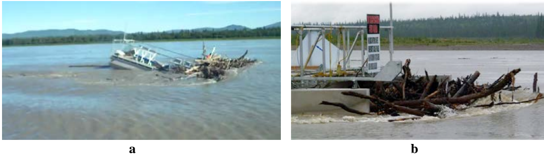
Figure 50. Debris accumulation on the bow of the 5 kW New Energy EnCurrent turbine barge on the Yukon River at Ruby, Alaska (Pelunis-Messier 2010) (a); debris accumulation in front of a 25 kW New Energy turbine barge on the Yukon River at Eagle, Alaska (photo credit: Alaska Power & Telephone) (b).
