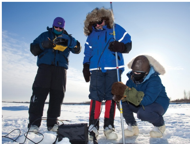
Figure 16. Tanana River under-ice current velocity measurements. UAF photo by T. Paris.
