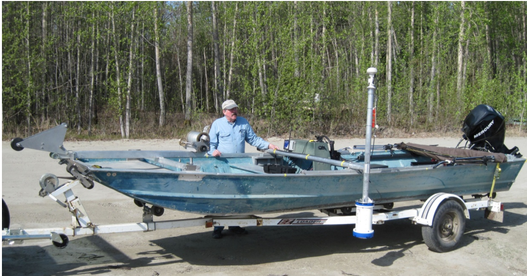
Figure B-1. Research boat on trailer with mounted ADCP & GPS.
