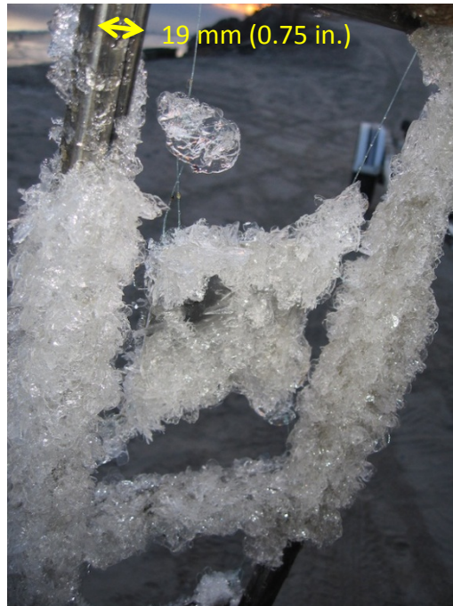
Figure 34. Frazil ice adhesion on nylon line and steel framework after about 5 hours of submersion in the Tanana River at Nenana (Oct. 22, 2009, air temp. -5 to +4^{\circ}\text{C} ). Photo credit: J. Johnson.
