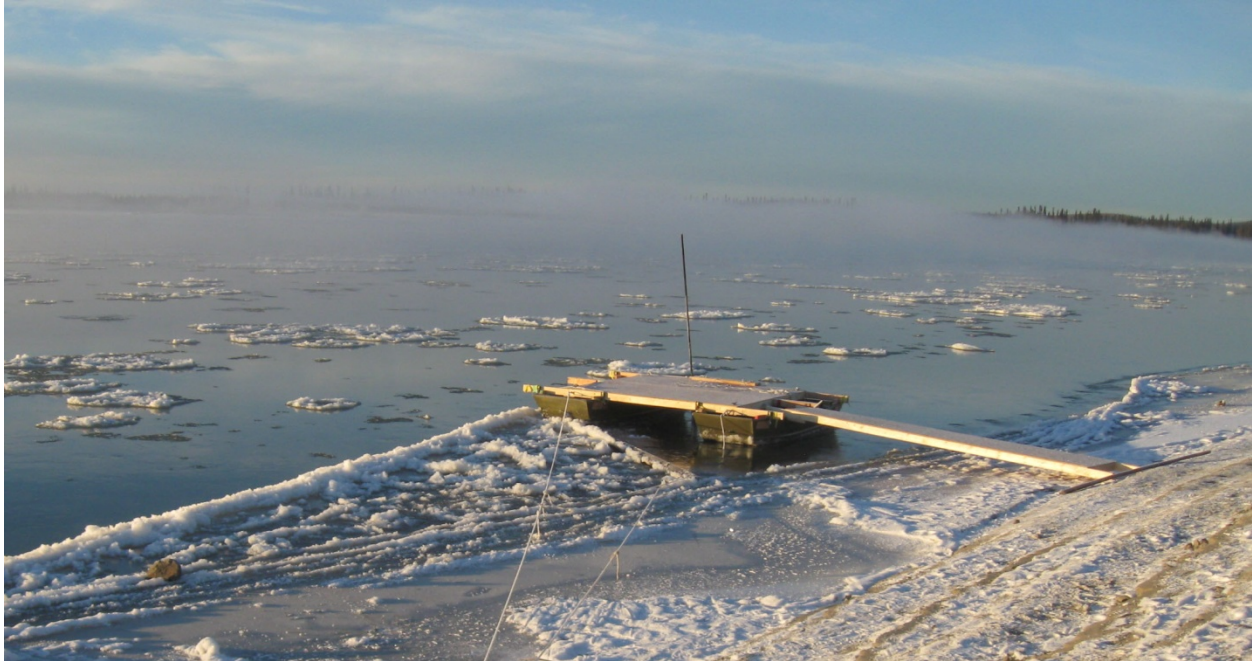
Figure B-7. Frazil ice growth platform deployed on Tanana River near Fairbanks showing vertical mild steel pipe on aft corner; river current is flowing from left to right. This image depicts the scene at 10 A.M. on 10/22/2010, just prior to removing the frazil samples in the frame on the aft end of the platform.
