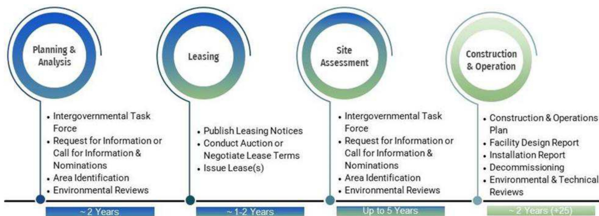
FIGURE 2 | BOEM regulatory roadmap for offshore wind development.
