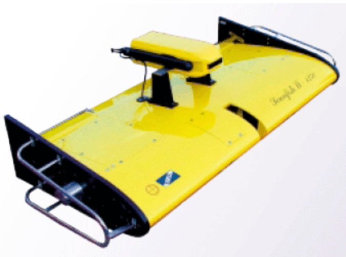
Figure 6-5: EIVA ScanFish II ROTV
