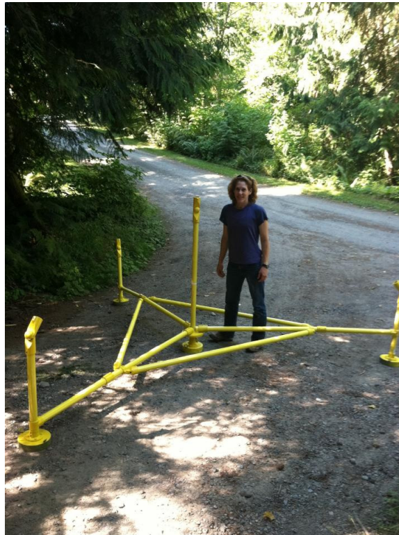
Figure 2.3. A star array mount prior to deployment. When deployed, a hydrophone is attached to the uprights at the center and the end of each of the arms of the mount.
