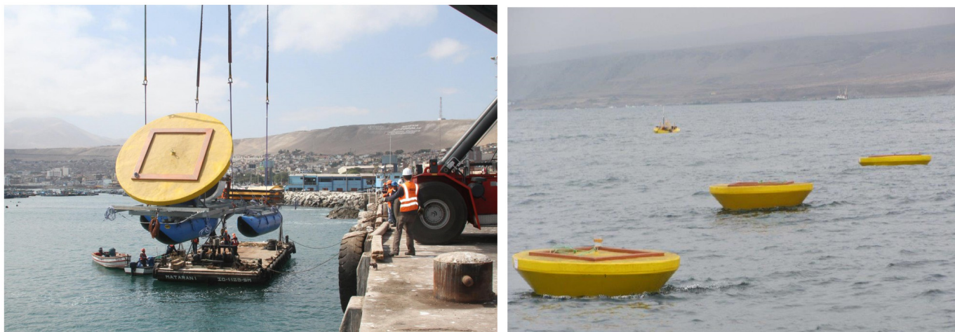
Figure 18. Panoramic view of point absorber water desalination device—Peru case study.
