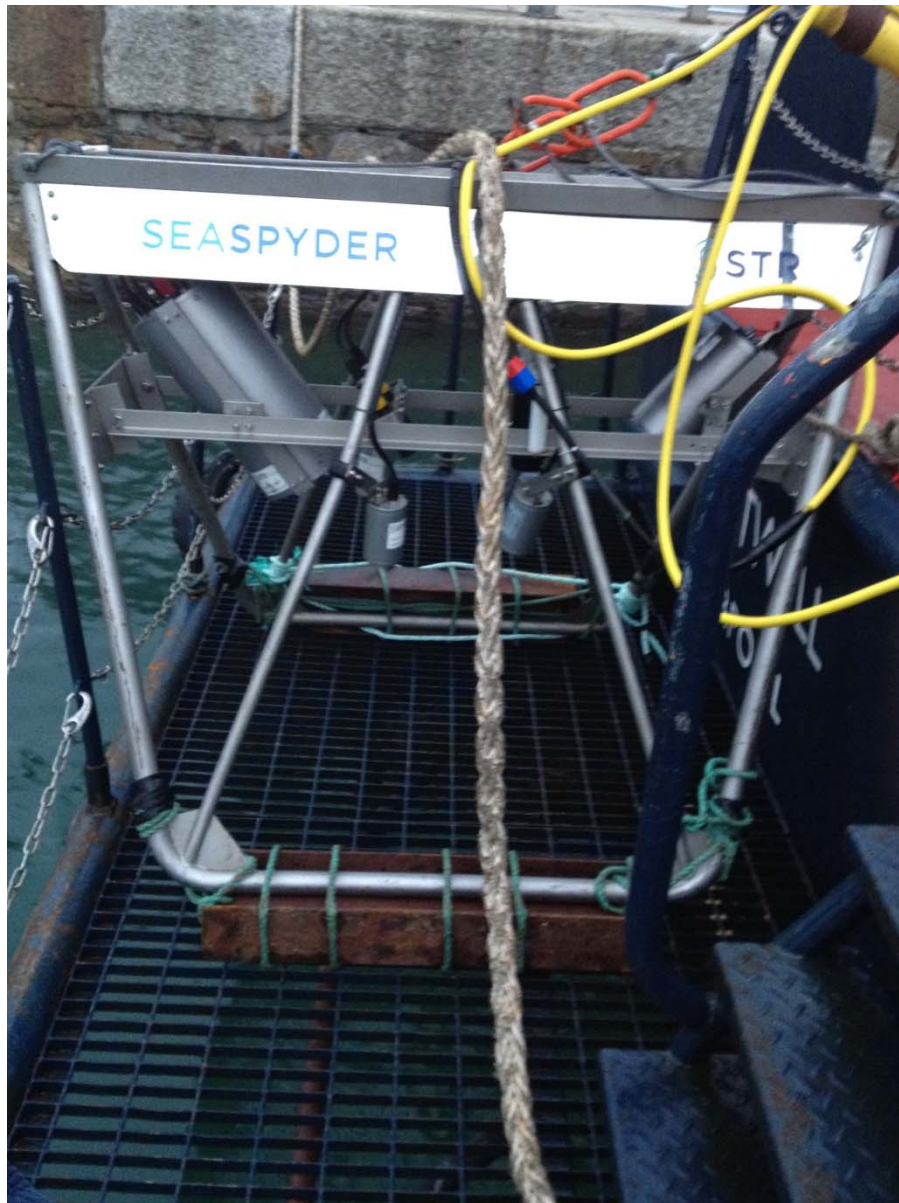
Plate 1. Seaspider dropdown camera system provided by STR.
