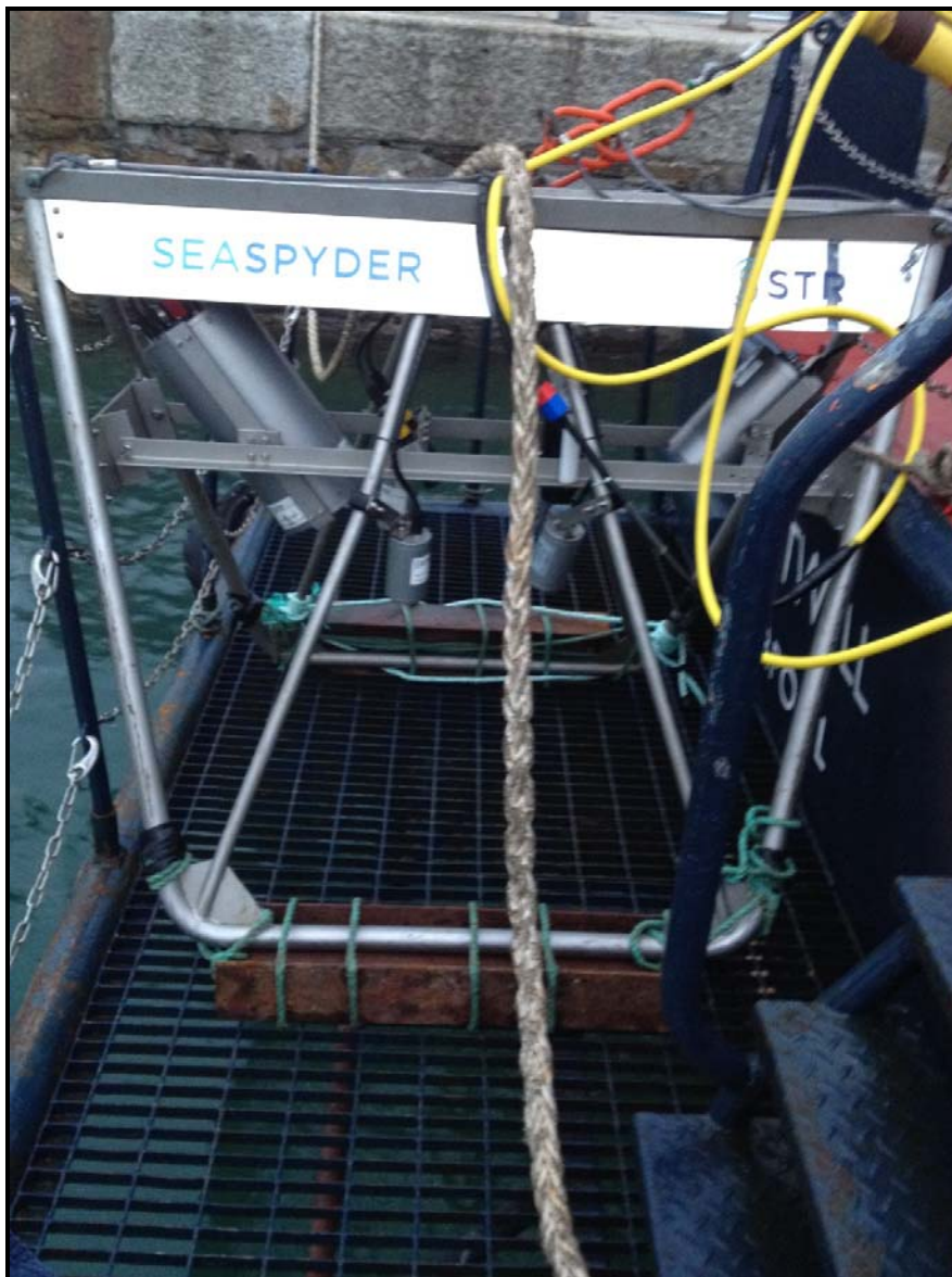
Plate 2. Seaspider drop down camera system provided by STR.
