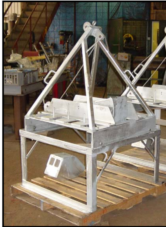
Plate 3. Mini-Hamon grab used for grab survey
