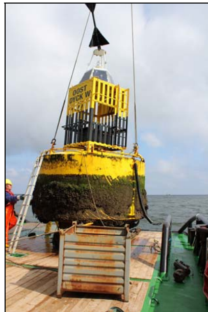
Figure 2. Oostdyck W buoy upon recovery, with a PoD (REF2) hanging from the side (right).
