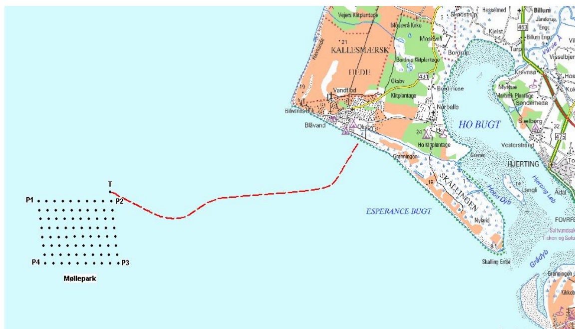
Figure 1. The offshore wind farm at Horns Rev and the cable trace to land at Hvidbjerg Strand. T marks the transformer platform.
