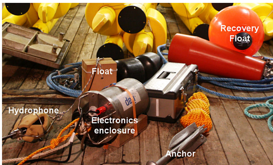
Fig. 3.2. Sound measurement buoy aboard M/V Tine Bødker, shortly before deployment (the hydrophone is still wrapped in protective foam)
