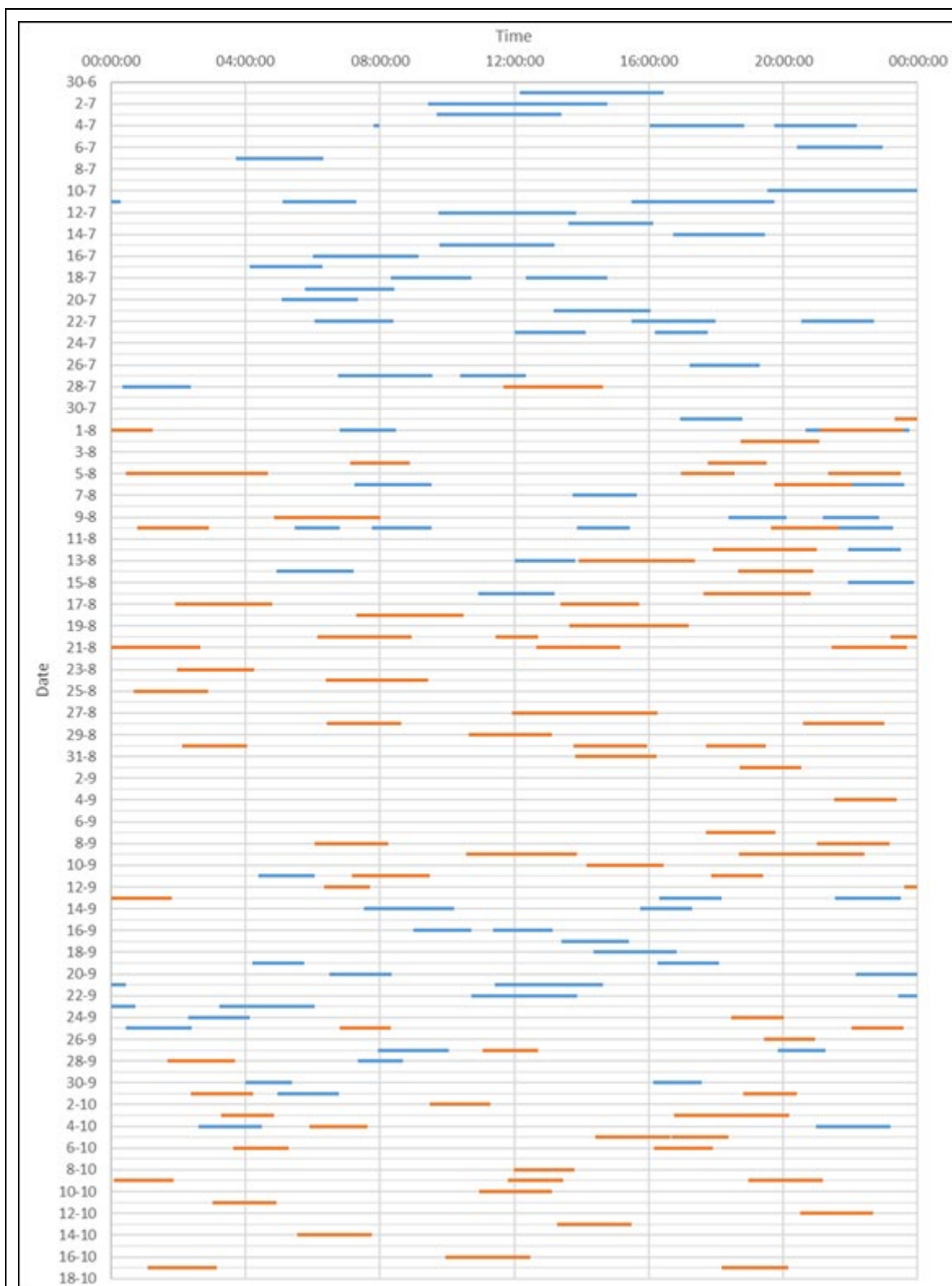
Figure I.1: Timing of pile driving activity in ZeeEnergie (orange) and Buitengaats (blue), 1 July – 17 October 2015. Bars show timing and duration of pile driving (see Annex 2 for details).
