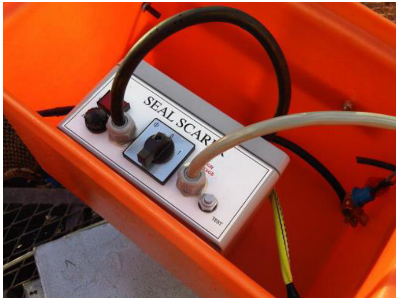
Figure C2. Lofitech control unit housed in a waterproof box.
