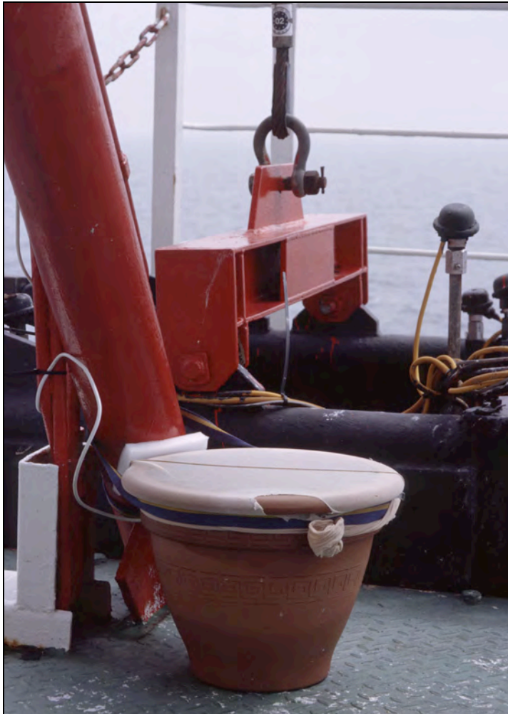
Microphone for automated sound recording on the platform. Photo: K. Krijgsveld
