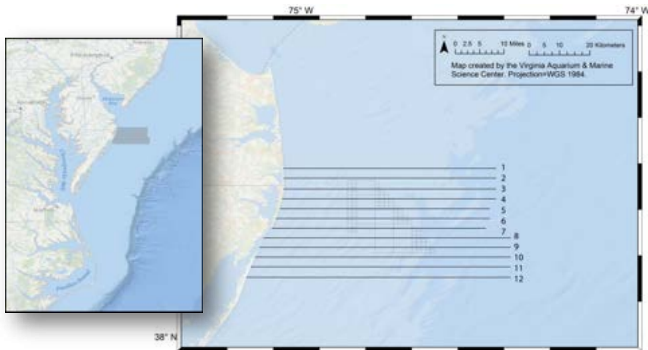
Figure 1: Survey lines numbered from north to south with the Maryland Wind Energy Area in the center of the survey area. The Maryland Wind Energy Area is shown in gray.
