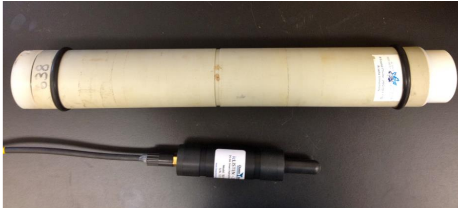
Figure 37: Image of a C-POD (top) and an icListenHF hydrophone (bottom) (Porskamp, 2013).
