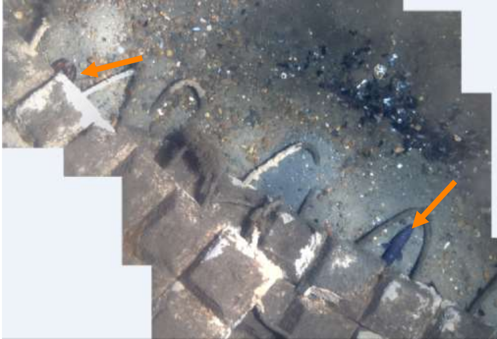
Figure 26. Example mosaic created from photographs taken by the float camera system in Year 1. The mosaics shows transition zones between gravelly and sandy seabed environments, shell hash (mostly blue mussel shells), and a portion of the concrete mat overlaid on sections of the buried cable. Also visible are fish and a lobster seeking cover under the concrete mat.
