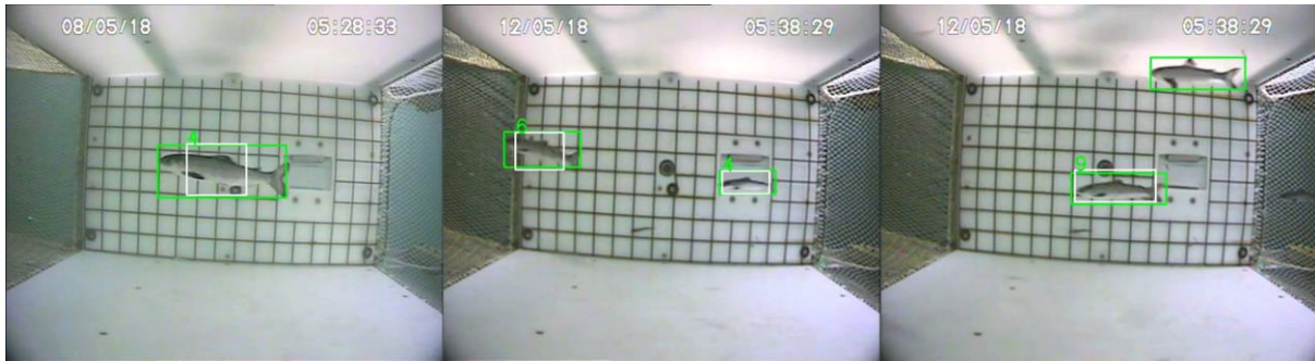
Figure 11: Fish detections in Video 1-5 using the FRCNN model. Detections from this CNN are shown as green boxes. The white boxes are from the DeepSORT tracking algorithm. The green number refers to the DeepSORT identification given to the tracked instance and does not necessarily reflect the count of instances.
