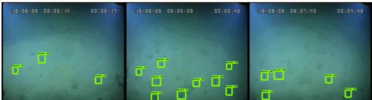
Figure 16: Potential Nephrops burrow detections in Video NB using the FRCNN model. Ideally the model should identify all hole-like objects in each frame for further post-processing. However, it is clear from these images that many of these have not been identified.
