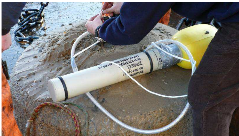
Figure 7: T-POD being attached to the anchoring system. The Kevlar line is reinforced with rubber tubing and a PVC foam float is attached at the top of the T-POD to increase the buoyancy.
