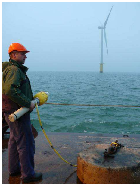
Figure 8: T-POD about to be deployed at position AT_5 in the OWEZ
