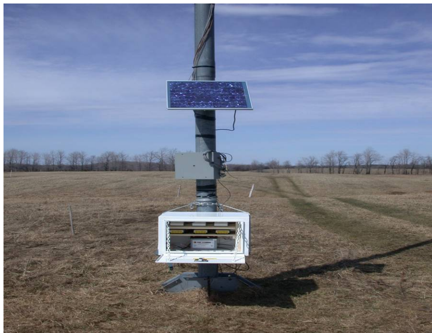
Figure 4. Waterproof boxes used to store acoustic detectors, data storage units, and a solar battery at ground-level and a 30 watt solar panel mounted to a meteorological tower (photo by D. S. Reynolds.)
