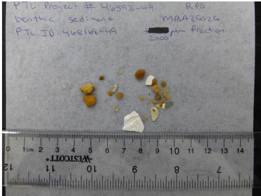
Figure B- 48. Photo of 2000 µm fraction of sediment from grab 2 of 2 at IA 2.
