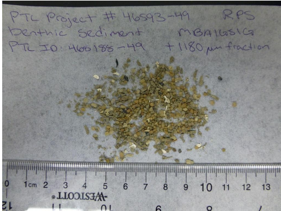
Figure B- 35. Photo of 1180 µm fraction of sediment grab 1 of 2 from IA 1.
