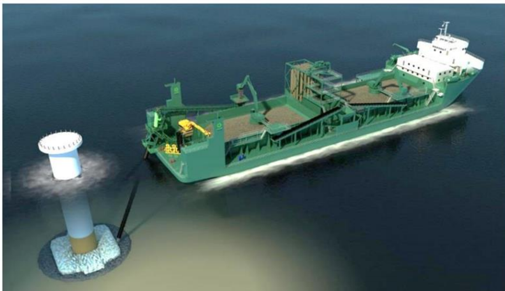
Figure 10: Example inclined fall pipe rock installation vessel showing the at deployment of the fall pipe next to a monopile.
