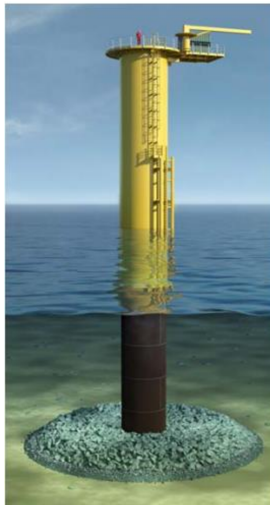
Figure 3: Typical monopile foundation with scour protection pad.
