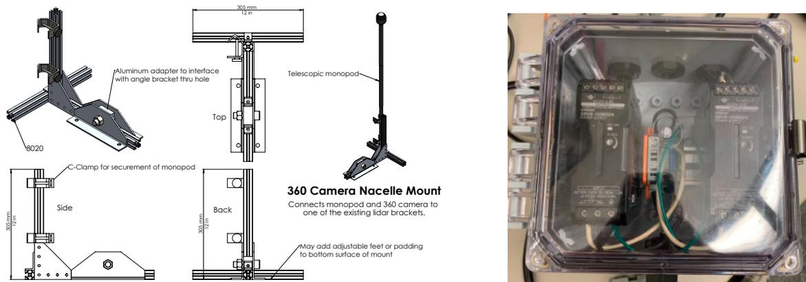
**Figure 14.** (left) Additional custom fixturing was designed and fabricated for mounting 360° camera on the nacelle. (right) Custom DC-DC power conversion assembly for powering on-blade modules from the turbine hub.
