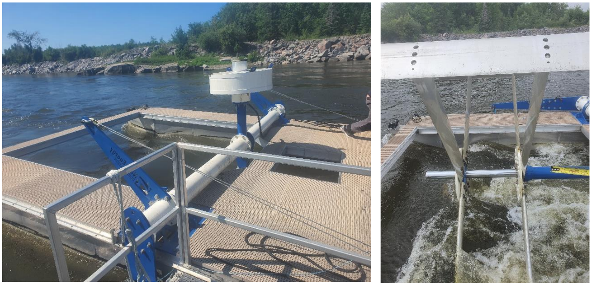
Figure 4: (Left) A detailed view of the VAHKT submerged under water at the CHTTC. The platform is designed for stability and precise positioning of the turbine for optimal data collection. (Right) Close-up of the VAHKT turbine blades.
