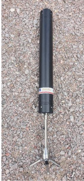
Figure 12: Vector 300 m ADV used in this study showing the 3 emitting beam which forms a sample measurement control volume under the instrument
