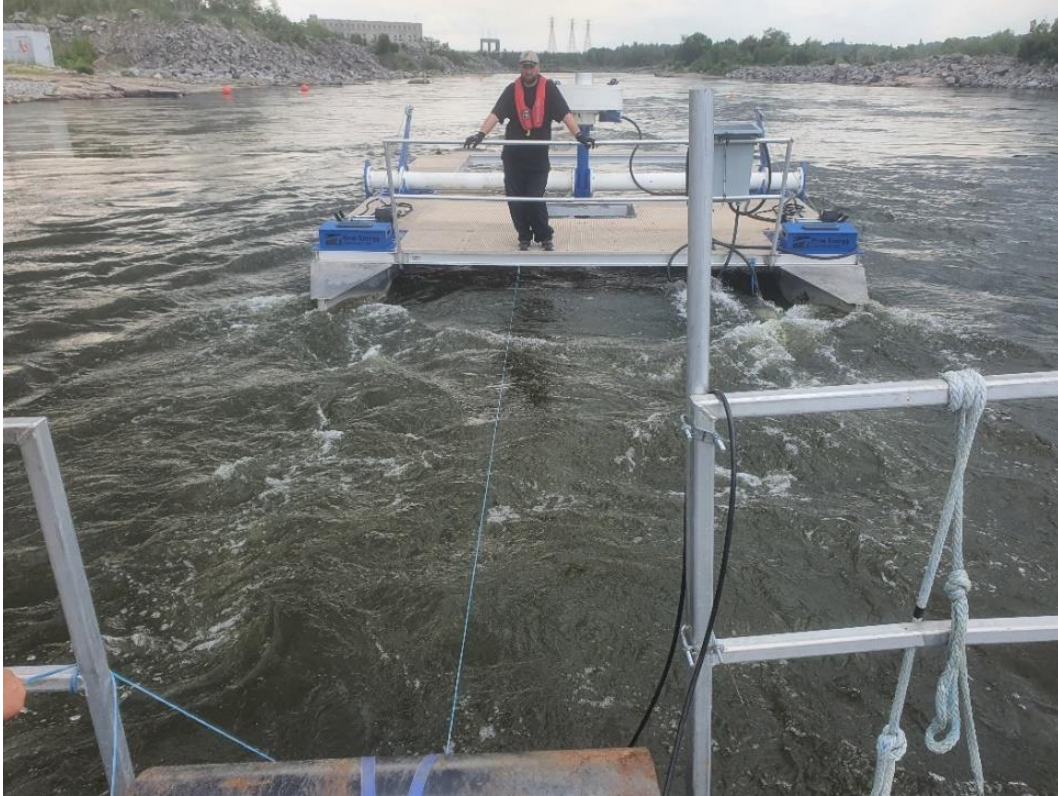
Figure 9: Data collection procedure at CHTTC, showing the floating pontoon platform equipped with a VAHKT. The setup includes a rope attached between the blue pontoon boat and the pontoon to measure precise distances downstream from the turbine. This configuration ensures accurate positioning for collecting flow velocity and turbulence data using the ADCP and ADV, facilitating comprehensive analysis of turbine performance and wake dynamics. Note pontoon vessel is always downstream of the turbine for safety.
