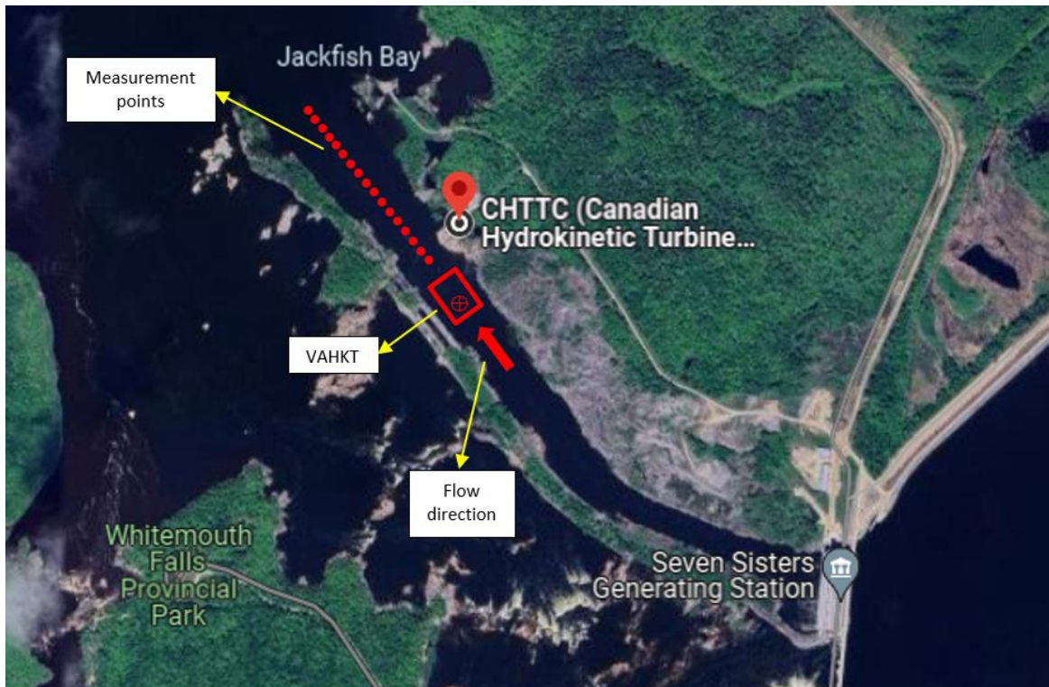
Figure 5: Aerial view of the CHTTC with annotations indicating the location of the VAHKT, flow direction, and measurement points. The red dashed line marks the downstream path where flow velocity measurements were taken using ADCP and ADV. The annotated flow direction arrow shows the water flow path from the Seven Sisters Generating Station towards Jackfish Bay, demonstrating the strategic placement for turbine testing and data collection.
