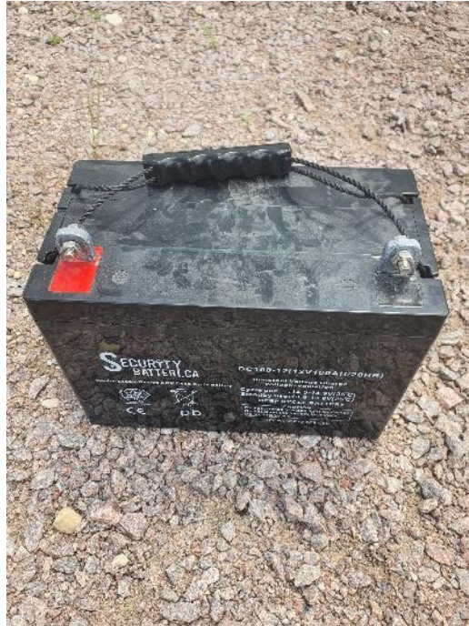
Figure 14: 12 V battery for power supply to provide power to the ADCP, ADV and laptop during testing
