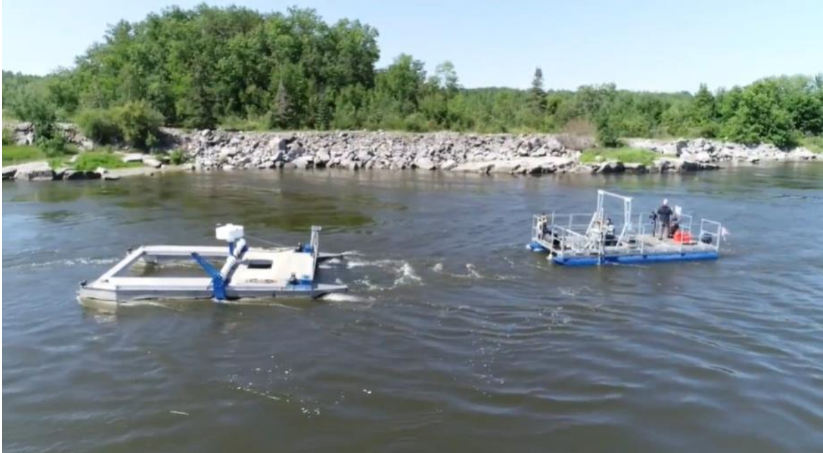
Figure 10: The setup for collecting TI and flow velocity measurements downstream of the VAHKT. The pontoon platform with the turbine is on the left, while the measurement equipment is positioned on the right platform. The rope system visible in the image is used to ensure precise distance measurements between the turbine and the measurement points, facilitating accurate data collection using the ADCP and ADV.
