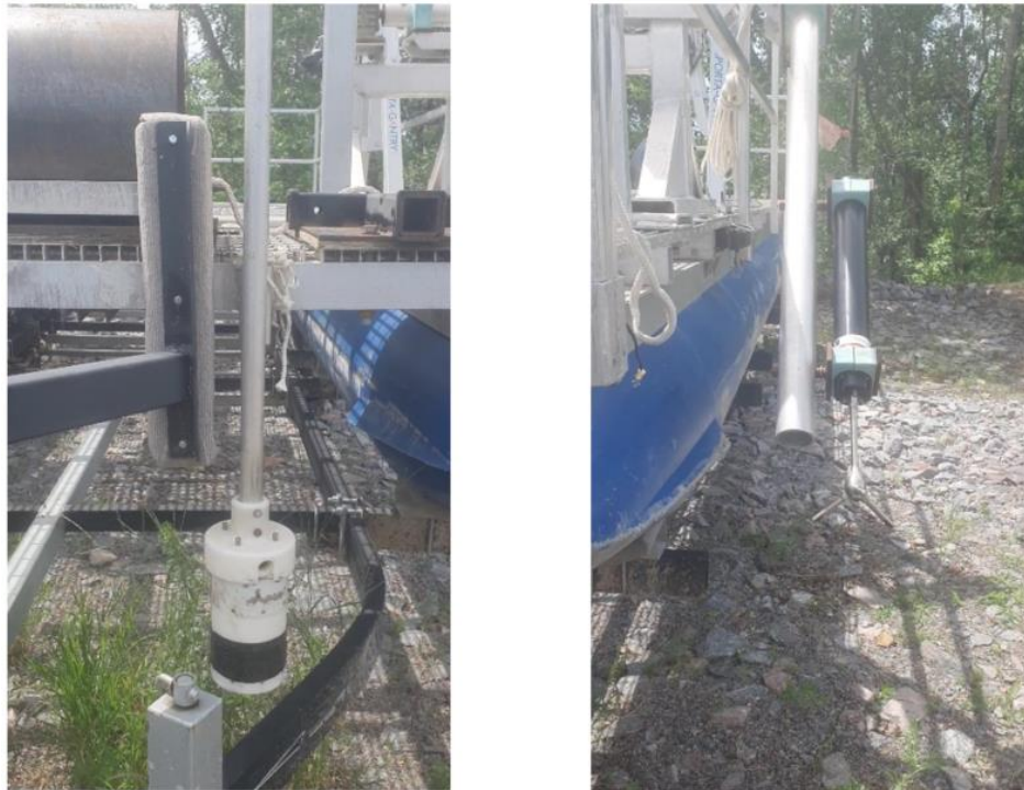
Figure 8: Deployment setup of measurement instruments on the floating pontoon platform at the CHTTC. (Left) ADCP mounted on the platform for comprehensive flow velocity measurements. (Right) ADV attached to an adjustable arm, used for high-frequency point velocity measurements. A Zodiac boat can also be used with similar mounts.
