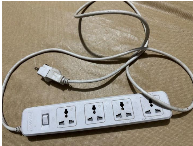
Figure 16: Grounded extension cord used on the vessel to provide power to instrumentation
