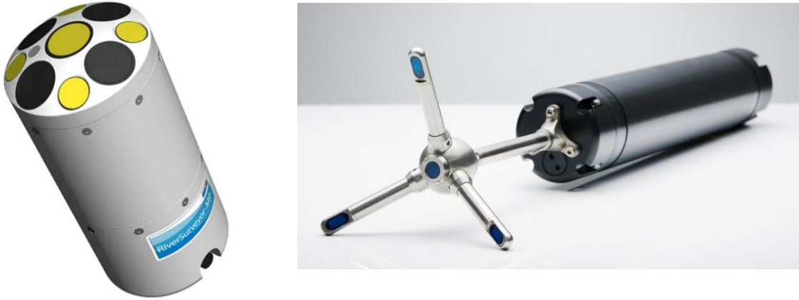
Figure 1: (Left) SonTek RiverSurveyor M9 ADCP, used for comprehensive flow velocity and discharge measurements across the entire water column (SonTek, 2013). (Right) Nortek Vector 300 m, utilized for high-frequency velocity measurements at specific points (Nortek, 2005).
