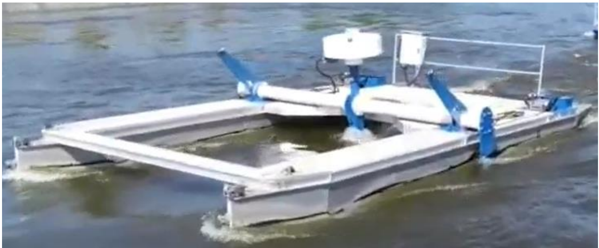
Figure 3: New Energy Corporation floating pontoon platform equipped with a 25-kW VAHKT being tested at the CHTTC. The turbine is mounted centrally on the platform, allowing for stable operation and precise measurements of flow characteristics and turbine performance in riverine environments. The setup facilitates in-situ testing and data collection for hydrokinetic energy research.
