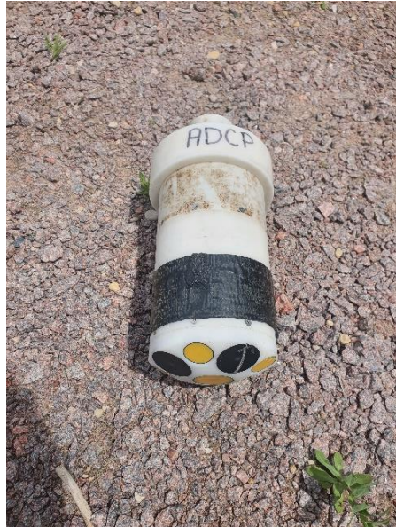
Figure 11: M9 ADCP instrument used in this study showing the 3 emitting beams and 3 receiving beams
