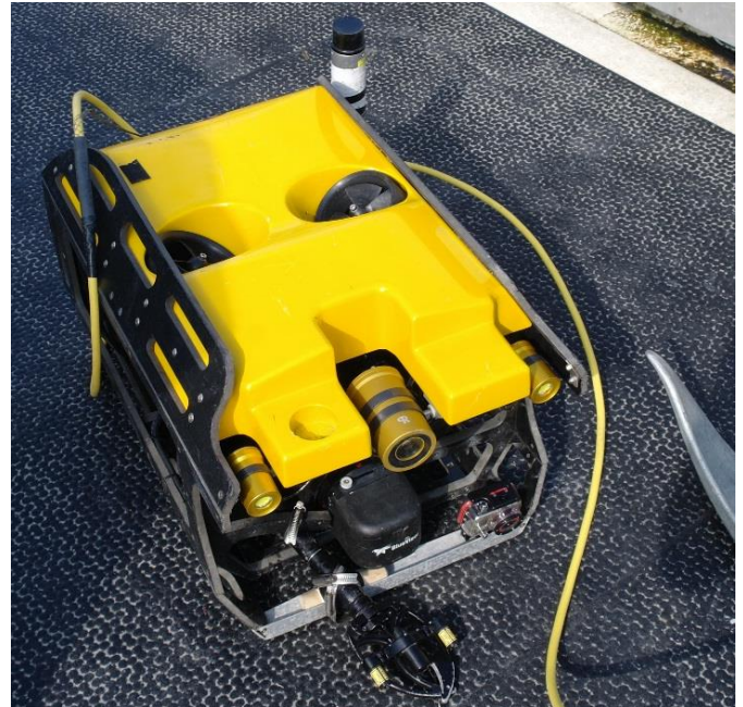
Fig. 3 ROV V4ST with attached grabber and laser pointer, GoPro, high-resolution camera and tether
