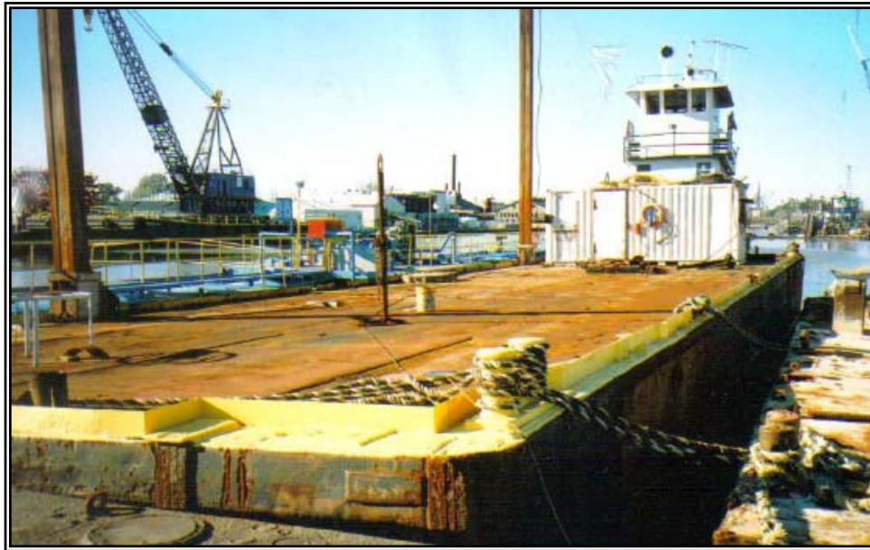
FIGURE 2-10 EXAMPLE OF A SPUD BARGE
