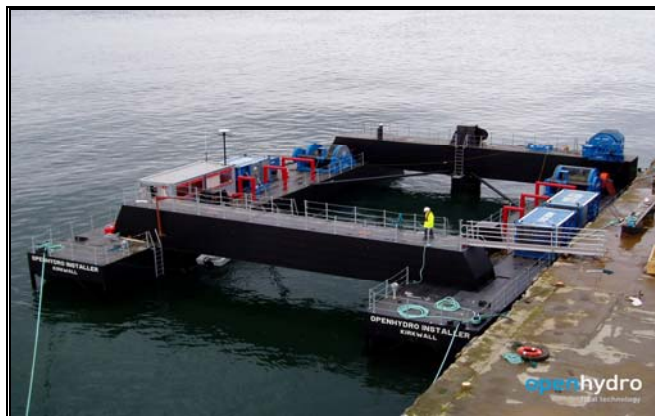
FIGURE 2-6 OPENHYDRO INSTALLATION BARGE
