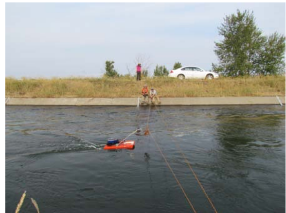
FIGURE 5. ADCP TEST MEASUREMENTS IN AUGUST 2013.
