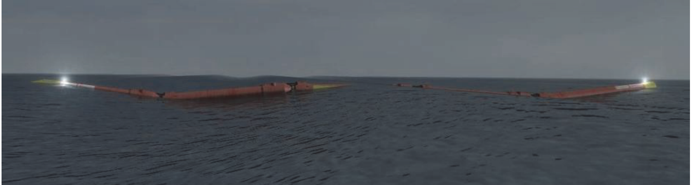
Figure 52: Pelamis warning lights
