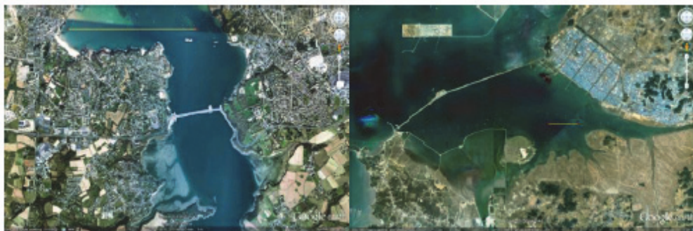
Figure 14: Tidal dams at Rance, France (left) and at Sihwa, South Korea (right) The yellow line on the photographs represents a distance of 2km.
