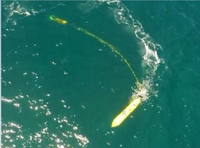
AUV-towed magnetometer: Aerial view (top), and side views (right)
